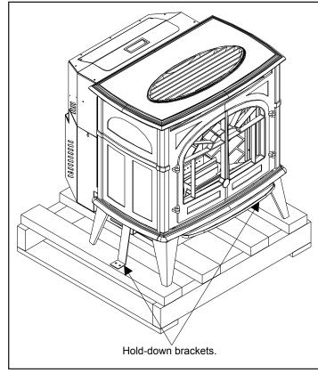
Figure 1: Removing Freestanding Stove From the Pallet.
